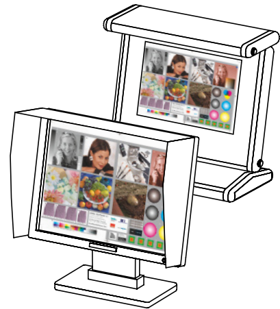
A profiled monitor with correctly set-up application software must show a good match with a proof in the light booth.
