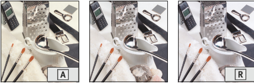
Image impression when the proof medium contains more optical brighteners than the printing standard being simulated (center: the original).
