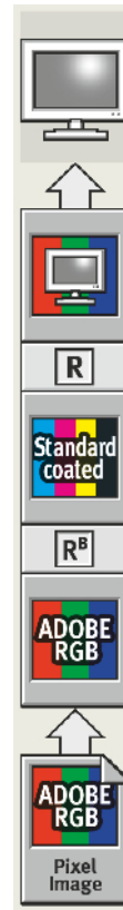
Color-management process with the standard coated soft proof of an RGB file
