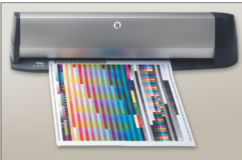
The i1 iSis from X-Rite is one of the fastest scanning measurement devices
